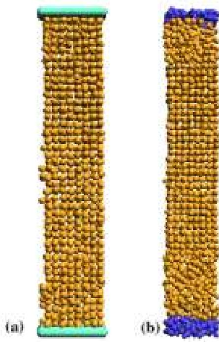
Figure 7.3: Snapshot of the Ar(001) slabs at  $P = 4.17$  GPa: (a) a sample with hard walls at  $T = 740$  K ( $T_m = 780$  K). (b) a sample with neon layers at  $T = 625$  K ( $T_m = 665$  K). Note the presence of premelting near the surface of the Ar-Ne sample.
