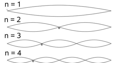
Vibration and standing waves: the fundamental and the first modes ( $n = 1, \dots, 4$ )
