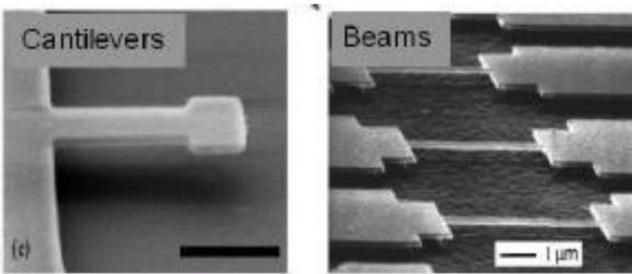
NEMS: Cantilevers of Aluminium Nitride (above left) [2] and Beams of Silicon Nitride (above right) [3].
