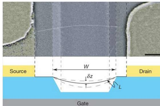
A doubly clamped Carbon Nanotube oscillator, device and geometry.[4]
